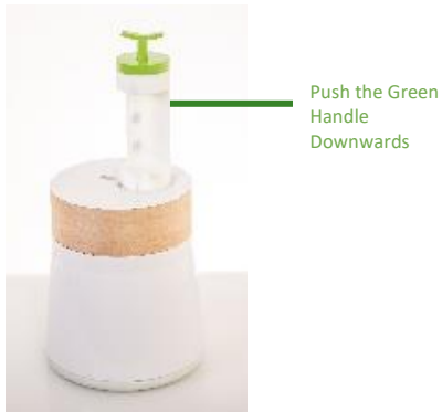
Figure 29: Pushing the Sample Drawer into the Device
