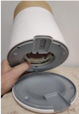
Figure 6: Pulling the Base Off the Device
