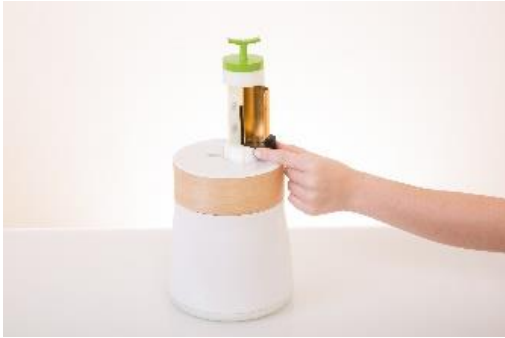
Figure 24: Sliding the Reflector into Sample Drawer
